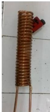
**Gambar 2.** Kondensor *dummy* tipe *helical coil*
