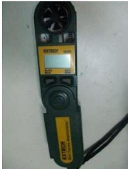
**Gambar 2.2 Mini Thermo-Anemometer Extech 45158**
