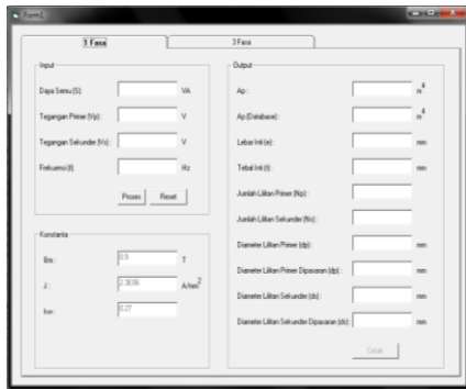
Gambar 4.2 Tampilan program perancangan transformator
