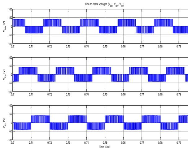
Gambar 4.4 Tegangan Output Inverter Fasa ke Netral
