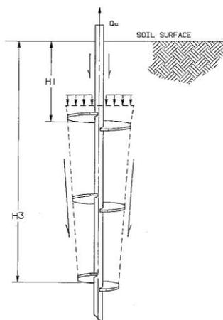
Gambar 2 Sketsa Mekanisme Konseptual *Cylindrical Shear Method* (Sumber: Lutenegro, 2009)
