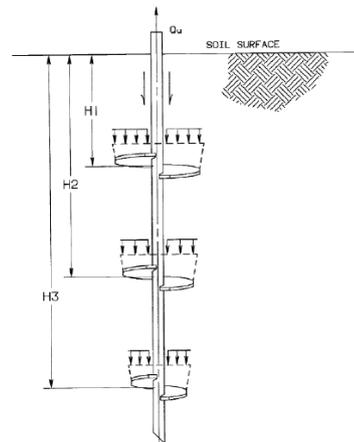
Gambar 1 Sketsa Mekanisme Konseptual *Individual Plate Method* (Sumber: Lutenecker, 2009)
