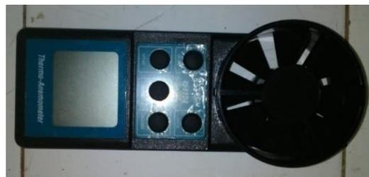
Gambar 4. Thermo-Anemometer Model 451104
