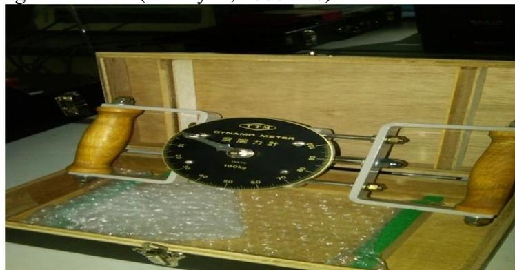
**GAMBAR 6: EXPANDING DYNAMOMETER**
