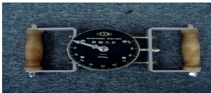
Gambar 1. *Expanding Dynamometer*
